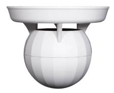
The SP3860W is a pendant speaker built-in 70V / 100V transformer. The 70V / 100V transformer technique reduces line losses on longer distance and allows easy parallel connection of multiple loudspeakers. The built-in 6" full range speaker driver is designed of wide frequency response 100-10 kHz, the multiple power taps of 7.5W, 10W, 15W, 20W, 30W & 60W could meet different applications varies from room size and ambient noise surroundings.
