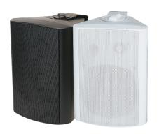
This wall mount speaker system has an active speaker with a 2x20W @8 $\Omega$  amplifier and a preamplifier to connect a balanced source line to a Phoenix connector or an unbalanced one to a RCA connector.
