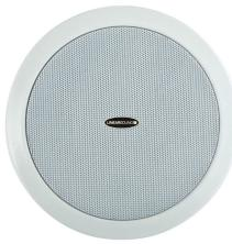
The PL249 is a ceiling speaker built-in 70V / 100V transformer. The 70V / 100V transformer technique reduces line losses on longer distance and allows easy parallel connection of multiple loudspeakers.
