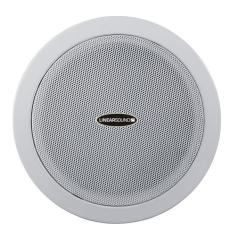
The PL166CF is a fireproof ceiling speaker built-in 70V / 100V transformer. The 70V / 100V transformer technique reduces line losses on longer distance and allows easy parallel connection of multiple loudspeakers.
