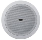
The PL2415CF is a fireproof ceiling speaker built-in 70v/100v transformer. The 70v/100v transformer technique reduces line losses on longer distance and allows easy parallel connection of multiple loudspeakers.
