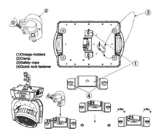
Screw one clamp each via a M12 screw and nut onto the Omega holders. Insert the quick-lock fasteners of the first Omega holder into the respective holes on the bottom of the device. Tighten the quick-lock fasteners fully clockwise. Install the second Omega holder.
