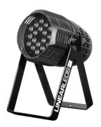
The PL183 is equipped with a heatsink. Therefore it does not require a fan, which makes this product very silent. It uses powerful LED, long life, low consumption and very bright. This projector, extremely light, is equipped with a switch for power on. It embeds the strobe functions, dimmer, effects of color changes, control by audio... It meets the international standard DMX512.
