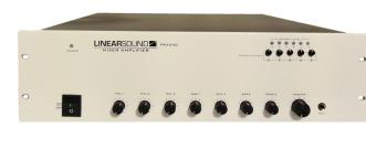
This amplifier - preamp offers for amplification part, a total power of 240W, 70V - 100V 4 and 16  $\Omega$  (100V line connections, which can be done on a terminal 5 zones whose commissioning is controllable on the front ). It also has a corrective tone 2 bands Bass -Treble, a general volume control on the front face and a bargraph level indication.
