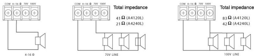
**Note :** Both the 4 - 16 ohms and 70V / 100V terminals cannot be used at the same time. Impedances indicated in the figures represent the total speaker system (load) impedances.
