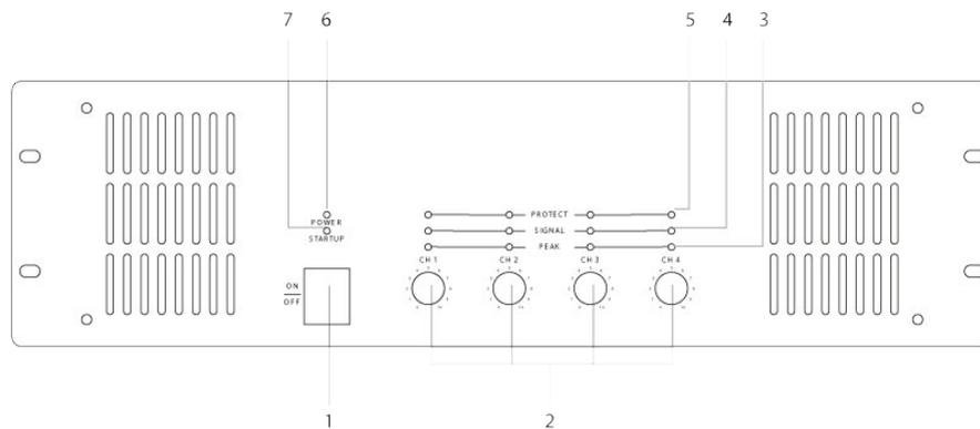
1. POWER SWITCH : On top of the opening Power. Press the end, power shut down
