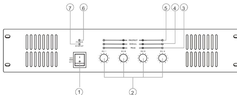
1. POWER SWITCH : On top of the opening power. Press the end, power shut down
