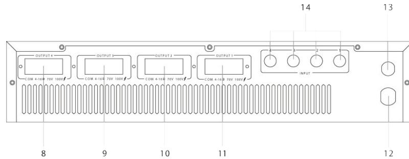
8. COMMON SPEAKER OUTPUT 4 : Connectors for 4~16 ohms or 70V and 100V speaker
