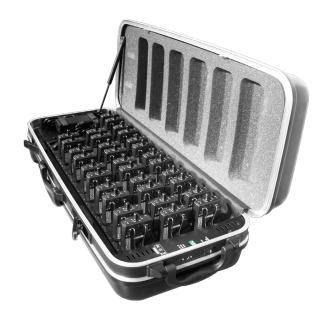
The smart charger, with its multiple simultaneous loads characteristics, is unique. It has 36 charging contacts and operates with a control system of the electronic charge and an automatic stop detector. It provides high efficiency: 3 to 4 hours to fully charge for 10 or 12 hours of operation with two rechargeable batteries.
