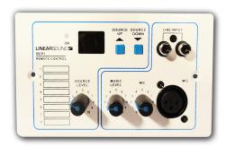
This remote control panel for MA88, permits to deport locally, in a selected area, level control of one of 8 selected sources or to select local inputs, Line and Mic (each has a level control) Visual control of active selection is made by the screen.
