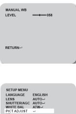
LEVEL (niveau) 0 - 255Specifies the R and B gain values for manual WB. Default setting is 58
