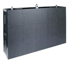
The P10SMD is a module for LED screen. It is equipped with trichromatic SMD 1R1G1B LED.
