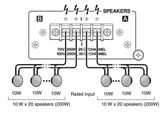
You may also connect speakers with different rated inputs to different channels or connect speakers with different rated input to the same channel, as shown below:
