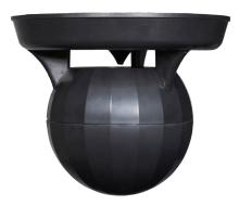
The SP3860B is a pendant speaker built-in 70V / 100V transformer. The 70V / 100V transformer technique reduces line losses on longer distance and allows easy parallel connection of multiple loudspeakers. The built-in 6" full range speaker driver is designed of wide frequency response 100-10 kHz, the multiple power taps of 7.5W, 10W, 15W, 20W, 30W & 60W could meet different applications varies from room size and ambient noise surroundings.
