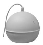
The SP206 is a pendant speaker built-in 70V / 100V transformer. The 70V / 100V transformer technique reduces line losses on longer distance and allows easy parallel connection of multiple loudspeakers. The built-in 5" full range speaker driver is designed of wide frequency response 130 - 14 kHz, the various power output 1.5W, 3W & 6W could meet different applications varies from room size and ambient noise surroundings.
