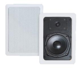
This 2 voices 40 watts speaker range, has a 8" boomer and a 1" tweeter Mylar. It is made in ABS with a metal grille with epoxy paint. It can be supply in 100V line or impedance bass. For inside use.
