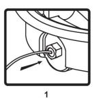
Pass the cable through the gland, making sure to keep a good sealing
