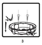
Screw the base of the speaker on the floor.
