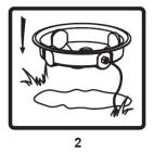
Position the speaker in the space provided and drill the mounting holes.
