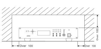
Keep the unit's all sides over 10 cm away from objects that may obstruct air flow to prevent the unit's internal temperature rise.
