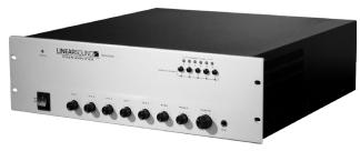
This amplifier - preamp offers for amplification part, a total power of 250W, 70V - 100V 4 and  $16\Omega$  (100V line connections, which can be done on a terminal 5 zones whose commissioning is controllable on the front)
