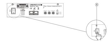
When the power switch is turned ON, the power stars and the indicator is on When the power switch is turned OFF, the power shuts off and the indicator is off.
