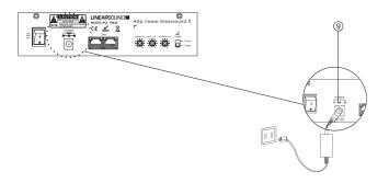
When the power supply of 24V DC starts, the unit can work normally. When the power supply of 24V DC stops, the unit will stop working.
