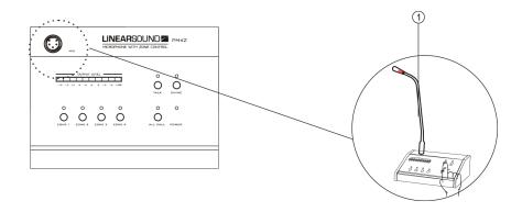
When input MIC, turn on the power, then press the call confirmation button, you can page to each zone independently or to all the zones. The volume could be adjusted by the volume control on the rear panel.
