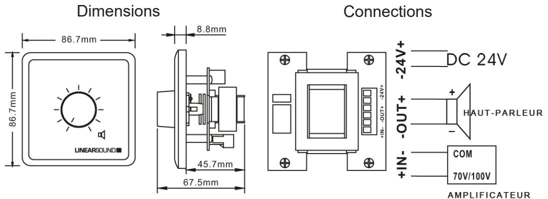
**Attention :** The usable wire should be IV and HIV type, whose diameter is 0.8-1.4mm, with cross-section acreage is 0.5-1.5mm<sup>2</sup> criterion wire .The signal is input into IN+ and IN- when playing music.
