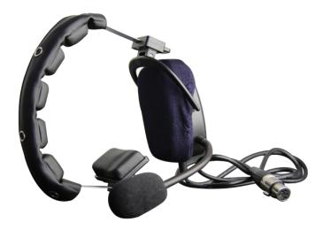
The H1 is a single-sided, medium-weight passive noise reduction headset with dynamic noisecancelling microphones. The headset has a noise reduction; suitable for use in a moderately noisy environment. The ergonomic moleskin-covered headband design distributes the ear cushion pressure evenly over the entire ear with no pressure points. An added advantage of this headset design is that it folds into compact form for ease of transport and storage.
