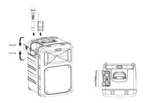
Open the box side of the hidden cover, to place the handheld transmitters.
